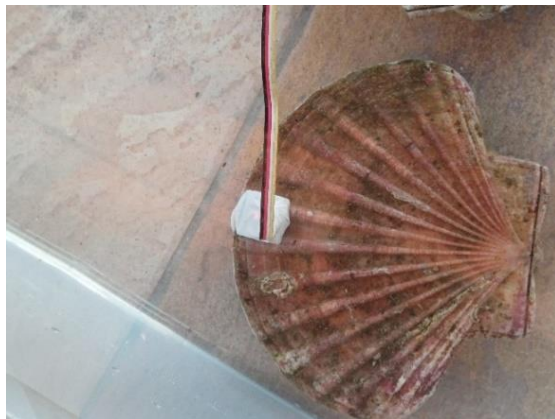
Figure 3. Hall sensor attached to the specimen of scallop ( Pecten jacobaeus , Linnaeus, 1758). A red light indicates that the sensor is working and the shells are closed.
